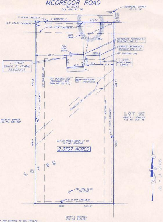
NOTE PIPELINE RIGHT-OF-WAY GRANTED TO SUN PIPELINE CO. FROM HERBERT T. HAYES, ET AL AS PER VOL 164, PG. 318.
