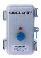
Every Singulair aerator is supplied with a prewired electrical control center for fully automatic operation. The control center is contained in a gasketed, lockable, corrosion resistant enclosure for safety and protection of components and wiring. Each control center is equipped with a resettable circuit breaker, on/off/automatic selector switch, red warning light, adjustable time clock and audible alarm. The
