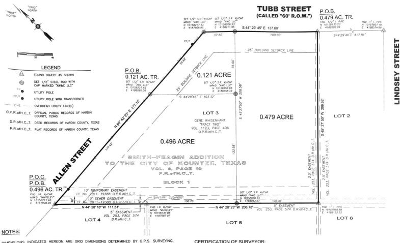
DIMENSIONS INDICATED HEREON ARE GRID DIMENSIONS DETERMINED BY G.P.S. SURVEYING, BASED UPON THE ALLTERRA CENTRAL, TRIMBLE V.R.S. R.T.K. G.P.S. NETWORK, REFERENCED TO THE (N.A.D. 83) TEXAS STATE PLANE COORDINATE SYSTEM, CENTRAL ZONE (4203) AND THE NORTH AMERICAN VERTICAL DATUM OF 1988 (N.A.V.D.88) USING GEOID MODEL "GEOID 18". COORDINATE, DISTANCE AND ELEVATION UNITS ARE U.S. SURVEY FEET.
