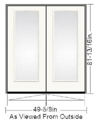
THERMA TRU, ENTRY DOOR, 4/0X6/8, RIGHT HAND INSWING ACTIVE, DOORSTYLE S140-LE, SMOOTH-STAR, SMOOTH-STAR, FLUSH NO/STILE LINES, FULL 1LT FLUSH, LOW-E GLASS, DOUBLE DOOR UNIT, DOUBLE BORE 2-3/8, NO BORE ON SECONDARY DOOR, 4-5/8" ROT PROOF BOTTOM JAMB, BRONZE WEATHERSTRIP, COMPOSITE ADJUSTABLE SILL WITH MILL DARK WOOD CAP FINISH, NO CASING NO CASING CASING, 6 RESIDENTIAL ZINC DICHROMATE HINGES, WHITE ALUMINUM W/FLUSH BOLTS ASTRAGAL, ACTUAL UNIT SIZE:49-5/8IN. X 81-13/16IN.
