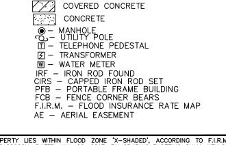
PROPERTY LIES WITHIN FLOOD ZONE 'X-SHADED', ACCORDING TO F.I.R.M. NO. 48201C0920M, DATED JAN. 06, 2017, BY GRAPHIC PLOTTING ONLY, WELLS LAND SURVEY DOES NOT ASSUME RESPONSIBILITY FOR EXACT DETERMINATION. BEFORE ANY DEVELOPMENT PLANNING, DESIGN, OR CONSTRUCTION IS STARTED, THE COMMUNITY, CITY, AND COUNTY IN WHICH SUBJECT TRACT EXISTS SHOULD BE CONTACTED, SAID ENTITIES MAY IMPOSE GREATER FLOOD PLAIN AND FLOODWAY RESTRICTIONS THAN SHOWN BY THE F.I.R.M. THAT MAY AFFECT DEVELOPMENT.
