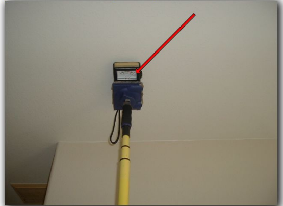
High moisture was detected in ceiling above entry area of the master bathroom linen closet There is evidence of water penetration in the attic at the type B vent to the HVAC unit.
