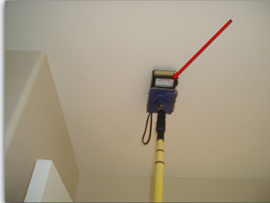
High moisture was detected in ceiling above entry area of the master bathroom linen closet There are cracked tiles at the front entry
