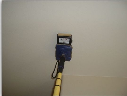
There is evidence of water penetration in the attic at the type B vent to the HVAC unit.
