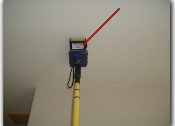
High moisture was detected in ceiling above entry area of the master bathroom linen closet
