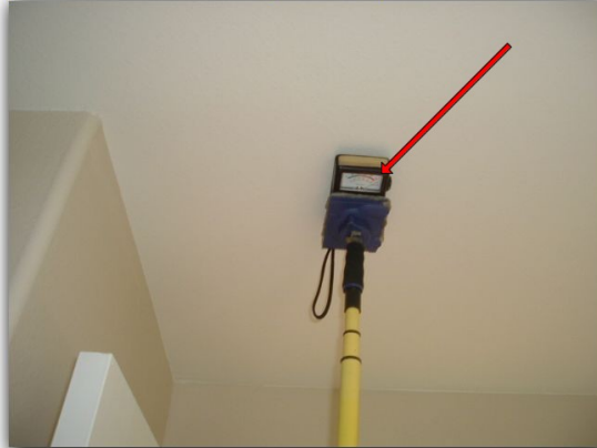
High moisture was detected in ceiling above entry area of the master bathroom linen closet There is evidence of water penetration in the attic at the type B vent to the HVAC unit.
