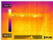
☑ Temperature differences and patterns associated with unconditioned air leakage observed when using the thermal camera on the attic access ladder cover.
