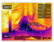
☑ Temperature differences and patterns associated with conditioned air leakage observed when using the thermal camera on the plenum.
