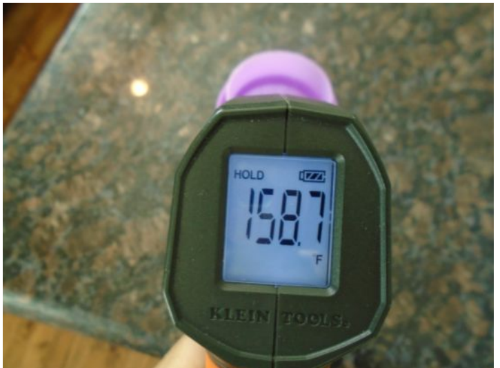
Microwave 30 second test indicated a 158.7 degrees temperature. Normal range is 125 -175 degrees.
