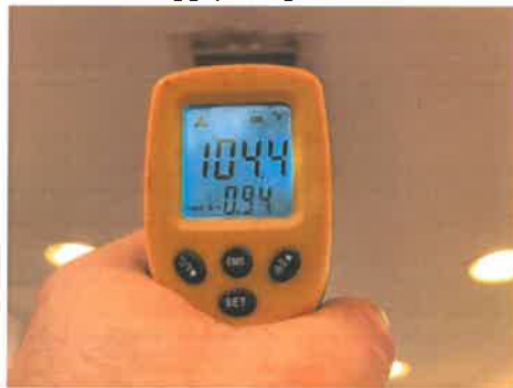
1st floor: hot air temperature
