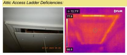
☑ Disappearing attic access ladder is not sealing properly at the attic.
