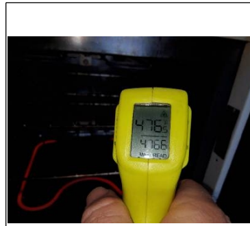
Oven temperature read 476° on the side of the unit, too hot
