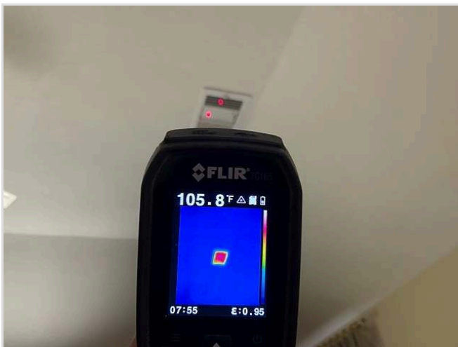
Thermal showing +100 degrees at supply register (den)
