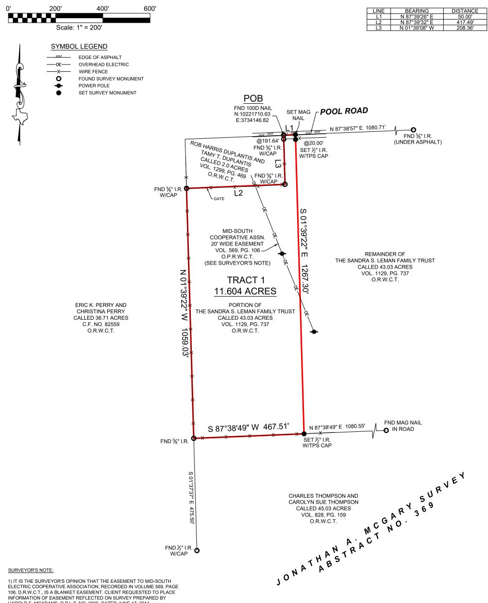
1) IT IS THE SURVEYOR'S OPINION THAT THE EASEMENT TO MID-SOUTH ELECTRIC COOPERATIVE ASSOCIATION, RECORDED IN VOLUME 569, PAGE 106, D.R.W.C.T., IS A BLANKET EASEMENT. CLIENT REQUESTED TO PLACE INFORMATION OF EASEMENT REFLECTED ON SURVEY PREPARED BY HAROLD E. MCADAMS, R.P.L.S. NO. 2005, DATED JUNE 17, 2014.
