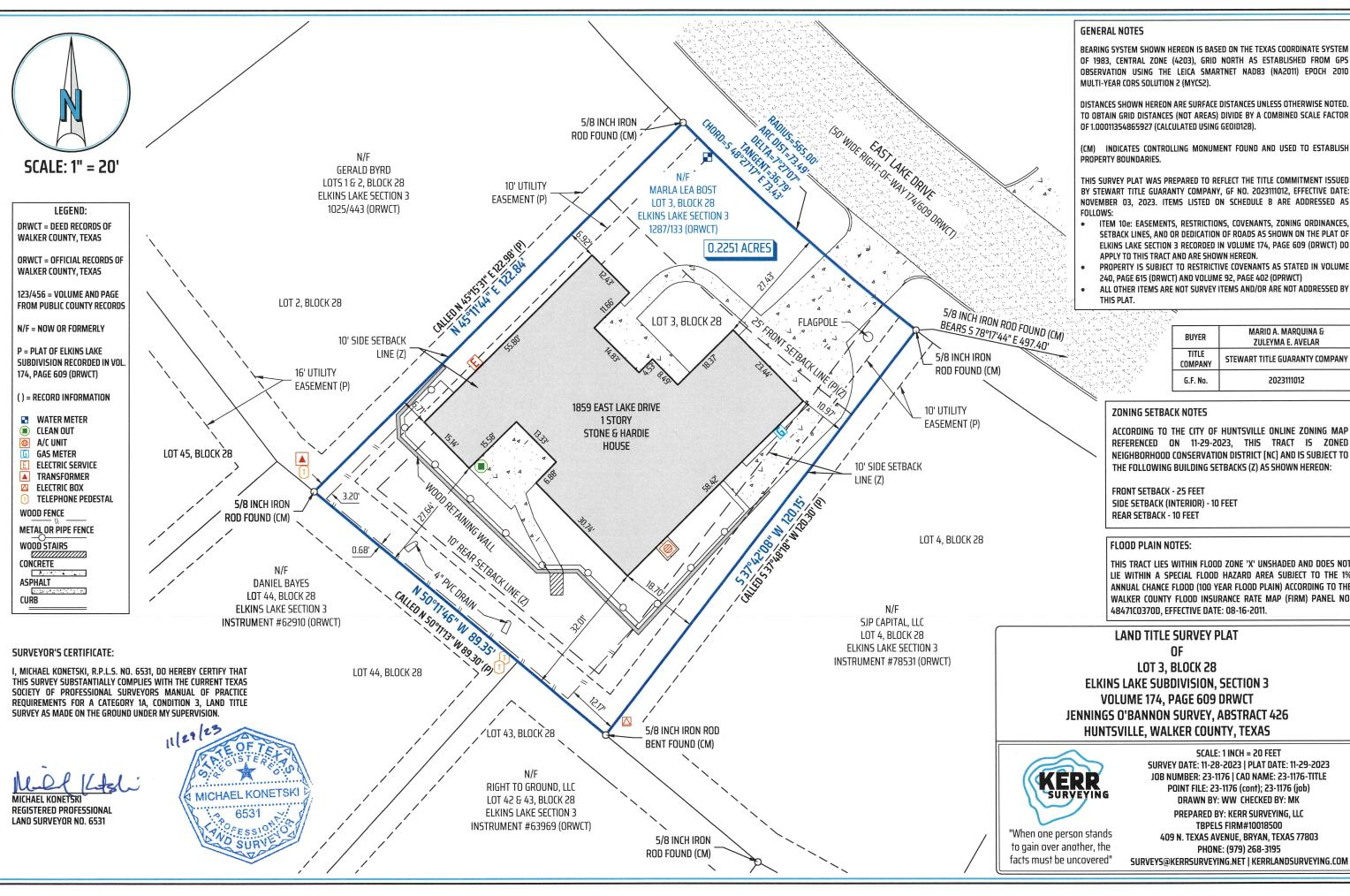
BEARING SYSTEM SHOWN HEREON IS BASED ON THE TEXAS COORDINATE SYSTEM OF 1983, CENTRAL ZONE (4203), GRID NORTH AS ESTABLISHED FROM GPS OBSERVATION USING THE LEICA SMARTNET NAD83 (NA2011) EPOCH 2010
