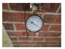
Static water pressure reading: 60 PSI (40-80 PSI is an acceptable static water pressure) Type of Water Pipping System: Copper
