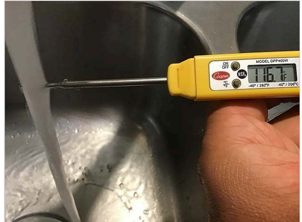
Hot water temperature reading at the kitchen sink (116.7 degrees)
