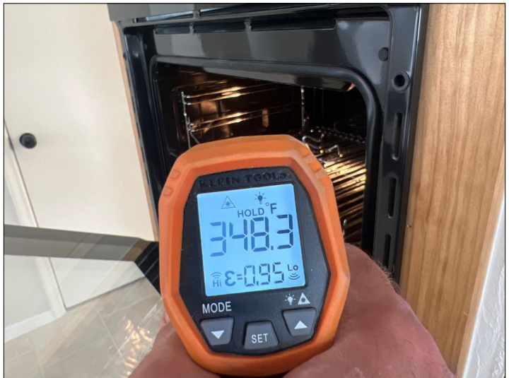
Oven Thermostat to Temperature Reading: 350F / 345-350F
