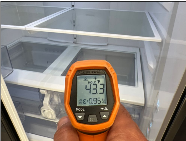
Overview of Refrigerator Cooling Temp.
