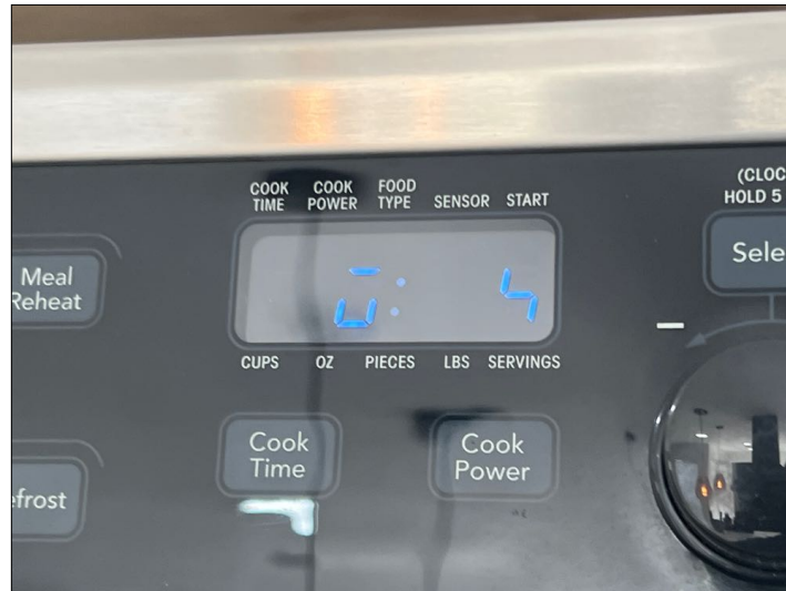
The clock numbers are damaged.
