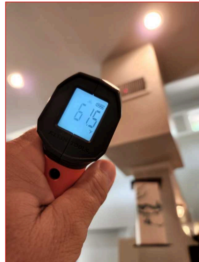
Supply temp 61.5 degrees. Main part of home.
