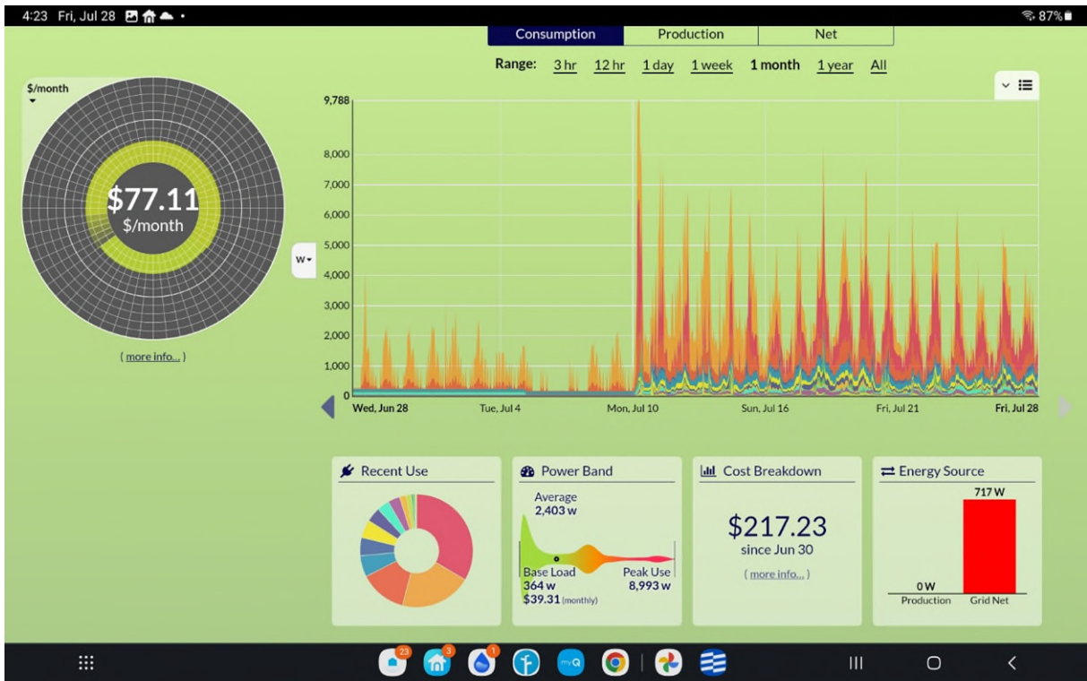
View of historical energy usage, note the peaks of when the AC systems are running. System also can project power usage costs.
