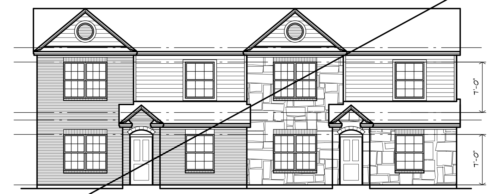
3 BLDG. C - FRONT ELEVATION 1/8" = 1'-0"
