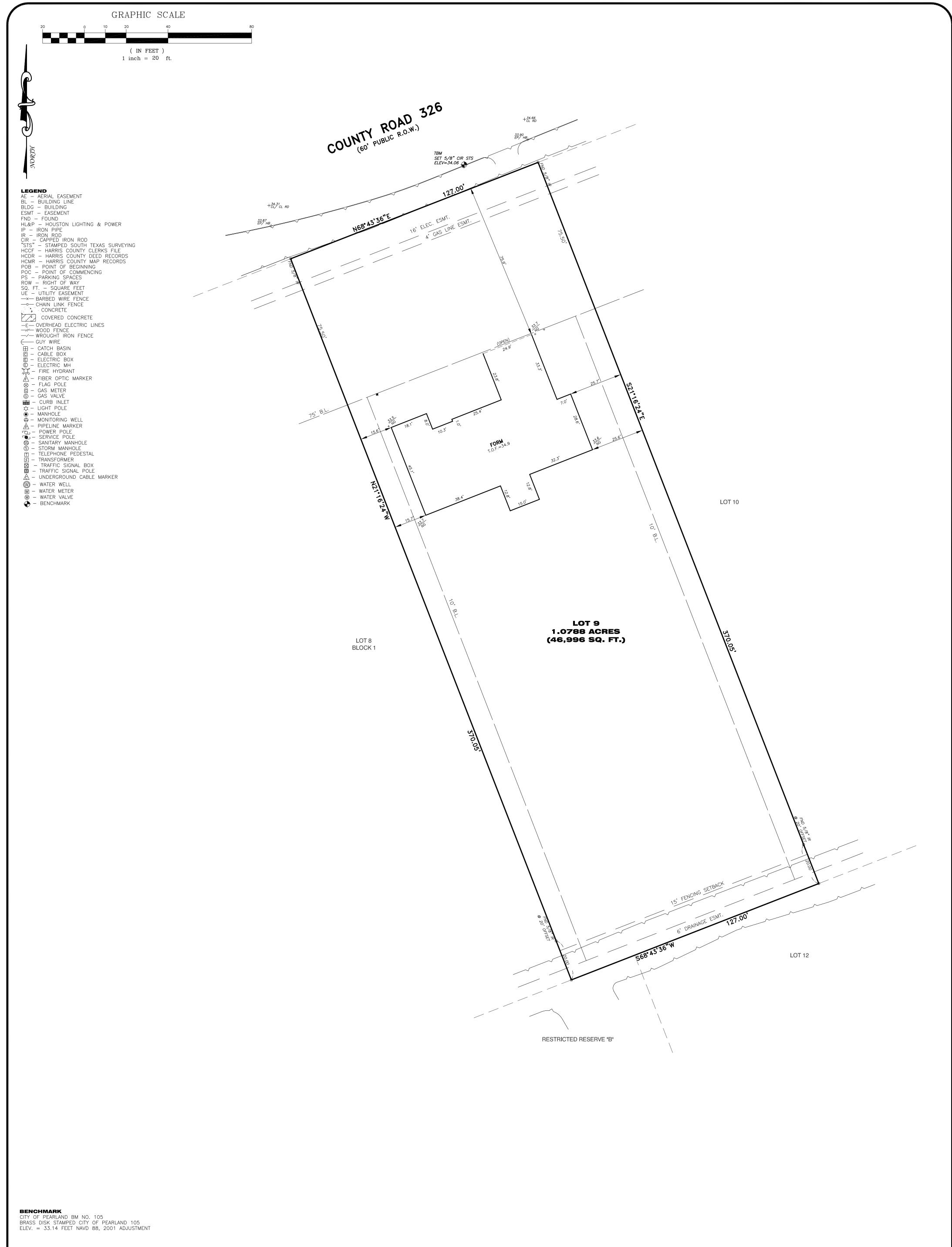
1. BEARING BASIS IS THE SOUTHEAST R.O.W. OF COUNTY ROAD 136 BEING N 68'43'36" E. 2. SURVEYOR DID NOT ABSTRACT PROPERTY. SURVEY BASED ON LEGAL DESCRIPTIONS SUPPLIED BY TITLE COMPANY, SURVEY AS SHOWN AND LEGAL DESCRIPTION AS PER AN ON THE GROUND SURVEY. EASEMENTS, BUILDING LINES, ETC., SHOWN ARE AS IDENTIFIED BY GF NO. CTH-FRW-CTT21739699LD OF CHICAGO TITLE INSURANCE COMPANY. 3. NOTHING IN THIS SURVEY IS INTENDED TO EXPRESS AN OPINION REGARDING OWNERSHIP OR TITLE.
