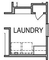
FIRST FLOOR PLAN OPT. #0152 LAUNDRY ROOM CABINETS
