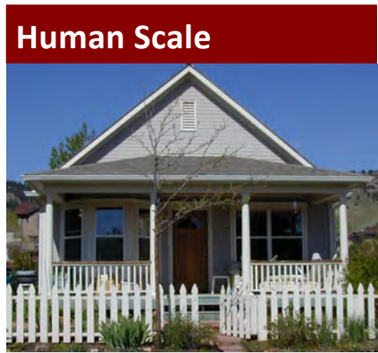
A sense of human scale is achieved when one can reasonably interpret the size of a building by comparing features of its design to comparable elements in one’s experience. Using building materials of a familiar dimension such as traditional brick or wood lap siding is an example, as is using windows, doors and porches of similar dimensions.
