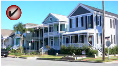
Locate a new building to fit within the range of setback dimensions seen in the block.
