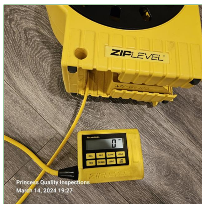
A. Item 18(Picture) Zip level spot check of foundation for level
