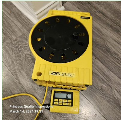
A. Item 1(Picture) Zip level spot check of foundation for level
