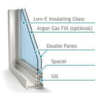
Double Glazed Window Structure
