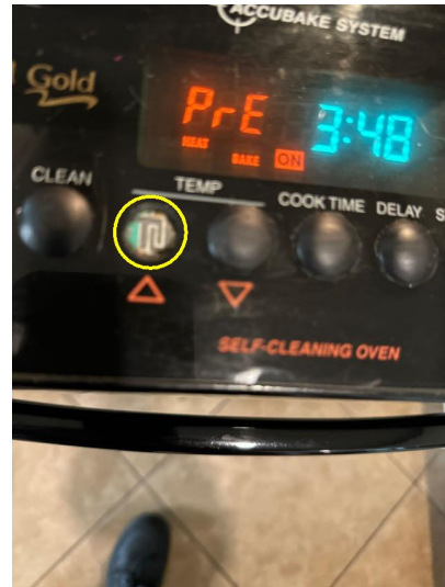
Temperature control button was worn.
