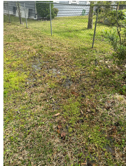
There was a wet area in the right front section of the yard and may be related to the septic system.
