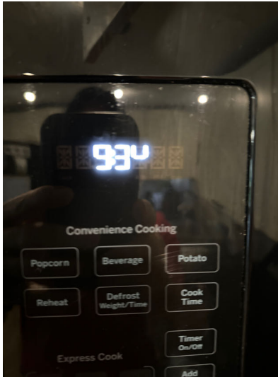
The digital display was missing pixels.
