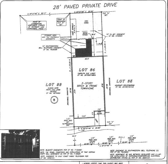
THIS PROPERTY IS AFFECTED BY THE 100 YEAR FLOOD PLAIM AS PER FIRM PANEL NO. 48201C 0835 L MAP REVISION: 05/18/05 ZONE AE BASED ONLY ON WISULL EXAMINATION OF MAPS INDICCURACES OF FEMA MAPS PREVENT EXACT DETERMINATION WITHOUT DETAILED FIELD STUDY
