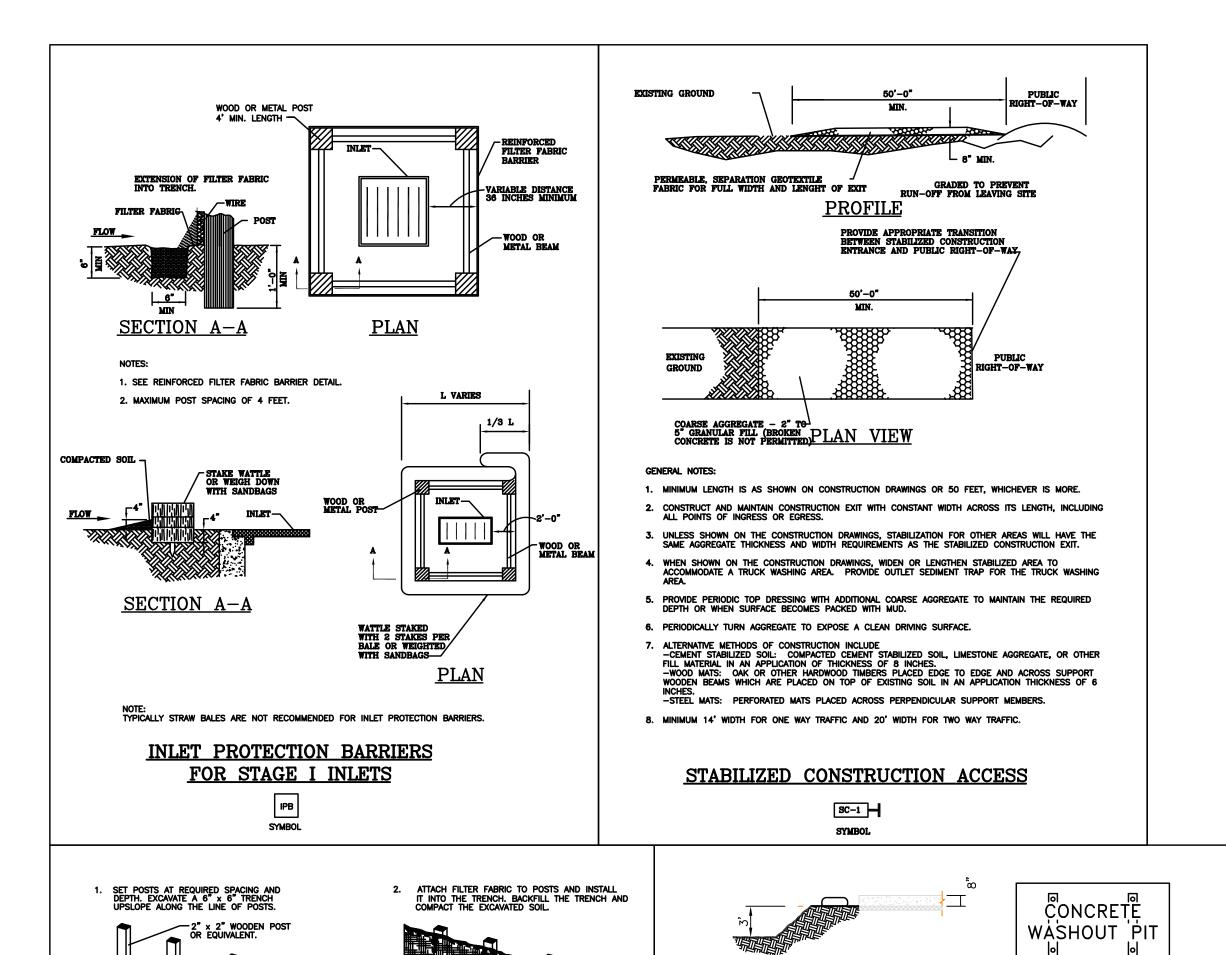
WHEN TWO SECTIONS OF FILTER FABRIC ADJOIN EACH OTHER, OVERLAP 6 INCHES AT THE POST, FOLD TOGETHER, AND ATTACH TO THE POSTS.
