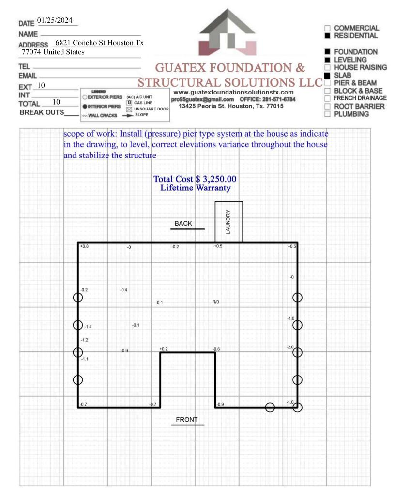
INTERIOR PIERS TO SUPPORT AT BEAMS OR USE 4"X4"X1,4"X16" LG ANGLE STEEL BEARIN INTERIOR PIERS NOT PLACED UNDER LOAD BEARING WALLS TO BEAR AT LEAST 1' FROM BREAKOUT
