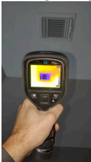
Air temperature measured at supply air vent.
