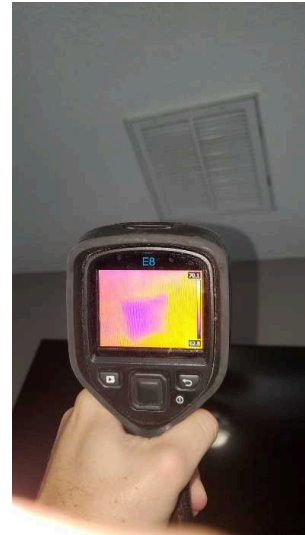
Air temperature measured at return air vent.
