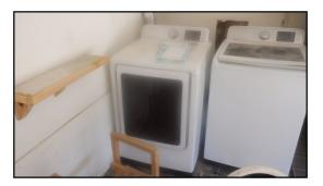
Unit did not function properly when tested on "Timed Dry" cycle. Unit was set to high heat but did not heat properly. Unit functioned normally under "Normal" setting.
