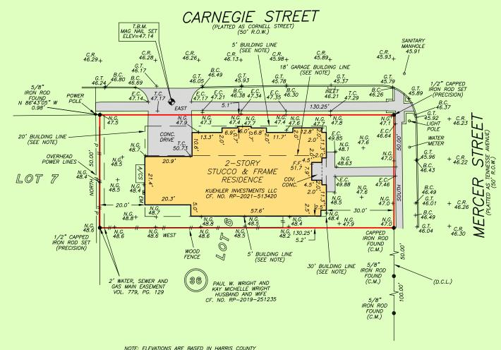
NOTE: ELEVATIONS ARE BASED IN HARRIS COUNTY FLOODPLAIN REFERENCE MARKER NO. 040135R ELEVATION=55.24 FEET NAVD88 2001 ADJ.
