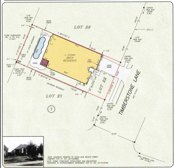
THIS PROPERTY DOES NOT LIE WITHIN THE 100 YEAR FLOOD PILAIN AS PER FIRM PANKE. NO. 48201C. 1150 L MAP REVISION: 06/18/07 ZONE X BASED ONLY ON VISUAL EXAMINATION OF MAPS. INACCURACIES OF FEMS MAPS PREVENT EXACT DETERMINATION WITHOUT DETAILED FIELD STUDY
