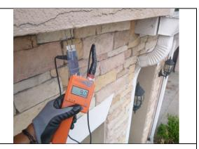
Low moisture and firm substrate (possible framing) below the front elevation overhang at the time of inspection. This is favorable.
