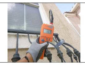
Low-to-mid moisture and firm substrate (possible framing) below the front elevation windows at the time of inspection. This is favorable.
