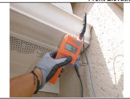
Low moisture and firm substrate (possible framing) below the roof junction at the time of inspection. This is favorable.
