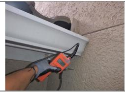
Firm substrate and Low moisture below the roof junction (probe 1) at the time of inspection. This is favorable.
