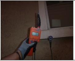
Firm substrate and low moisture below the right elevation window at the time of inspection. This is favorable. It is suggested to reseal all side elevation windows, accent bands, flashings, and penetrations (i.e., electrical boxes) at this time and every 2-3 years.
