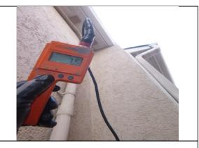
Firm substrate and low moisture noted at the probed location (several feet below the roof junction/small parapet wall) at the time of inspection. This is favorable.
