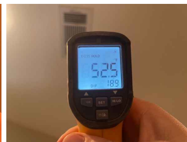
Unit 2: Photo of condenser data plate, Photo of evaporator data plate, Photo of return air temperature, Photo of vent temperature Delta T result: 19 degrees
