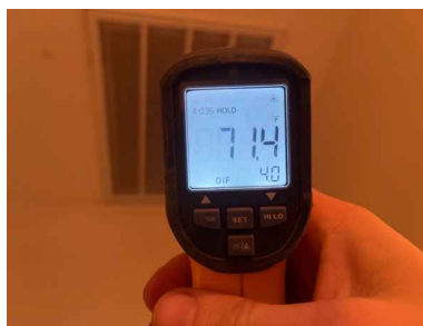
Unit 2: Photo of condenser data plate, Photo of evaporator data plate, Photo of return air temperature, Photo of vent temperature Delta T result: 19 degrees
