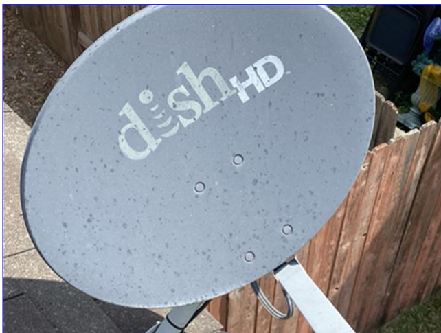
C. Item 3(Picture) Hail damage
