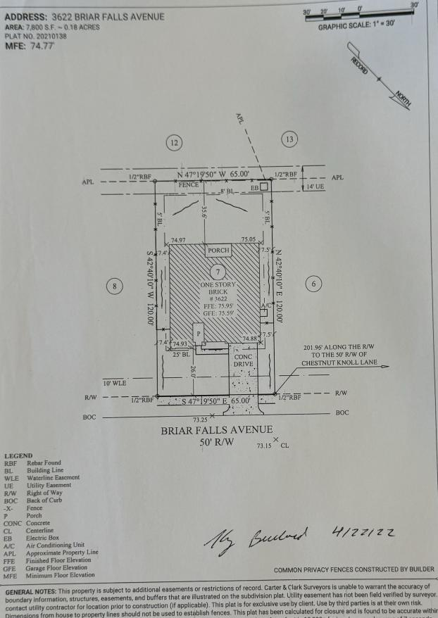
Dimensions from house to property lines should not be used to establish fences. This plat has been calculated for closure and is found to be accurate within one foot in 10,000+ feet. The field data upon which this plat is based has a closure precision of one foot in 10,000+ feet and an angular error of 7 seconds per angle point and was adjusted using the compass rule. Equipment used: Leica TS13 Robotic Total Station.
