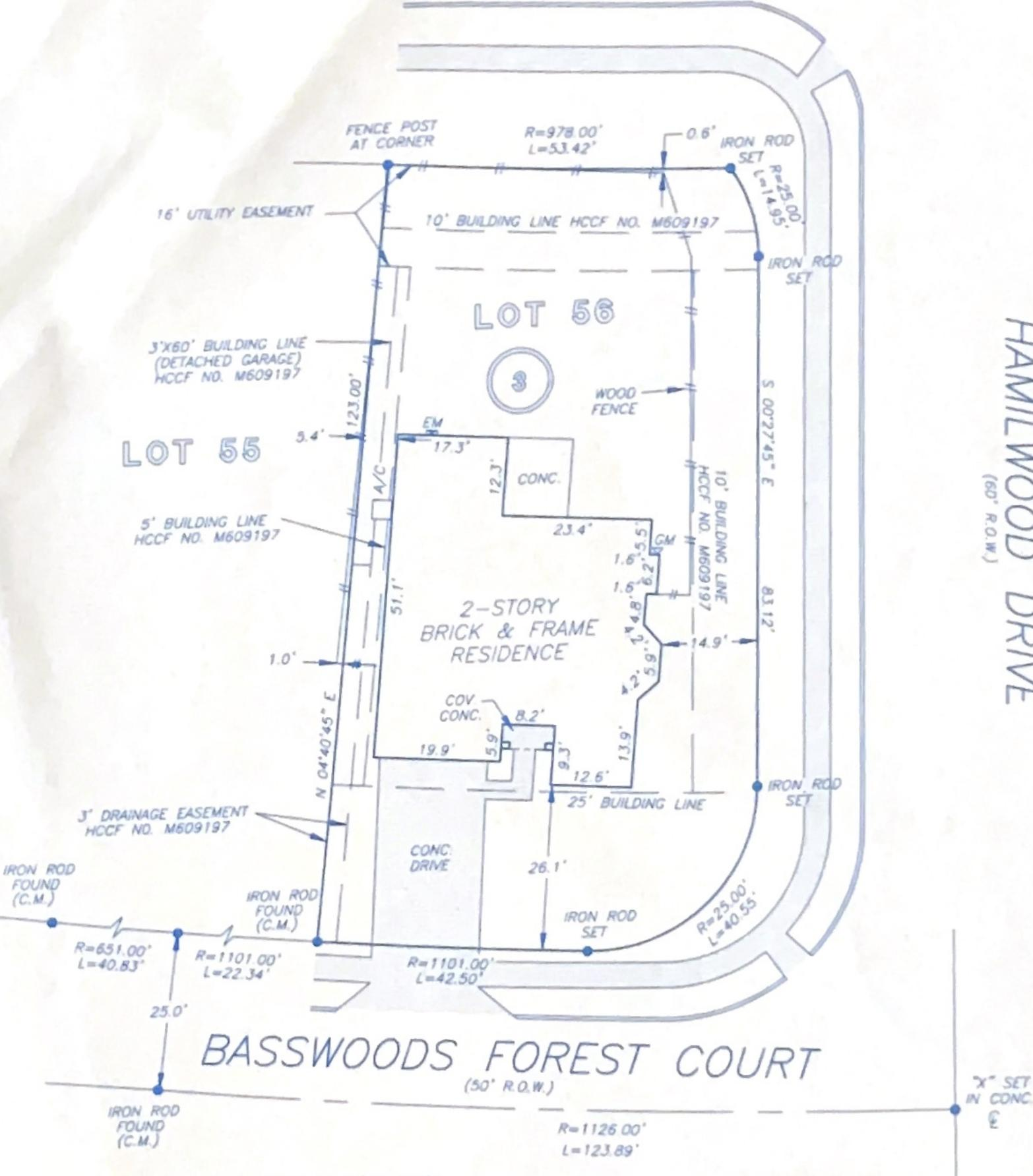
NOTE: BUILDING SET BACK LINE FOR RESIDENCE IS 20° IN WIDTH ALONG THE FRONT PROPERTY LINE(S) FOR LOTS LOCATED ON A CUL-DE-SAC OR 25° IN WIDTH ALONG THE FRONT FOR LOTS LOCATED ON THE STRAIGHT SECTION OF A STREET, AS PER HCCF NO. M609197.
