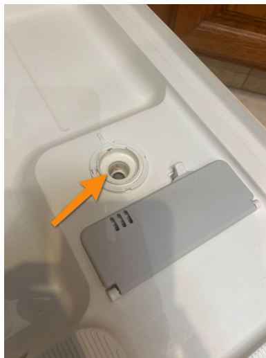
Rinse-Aid Cap Missing
