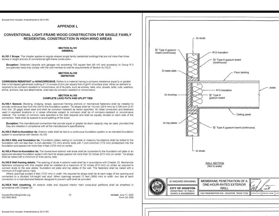
AL103.7 Floor-to-floor tie. Upper-level exterior wall studs shall be aligned and connected to the wall studs below with tie straps placed a maximum of 32 inches (813 mm) on center and connected with a minimum of 6 eight penny nails per
