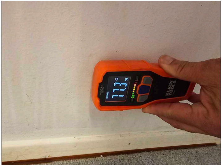
Checked water stain with a moisture meter and found it to be at a high moisture level. Unable to determine condition of the underlying materials. Mainly at - rear middle bedroom
