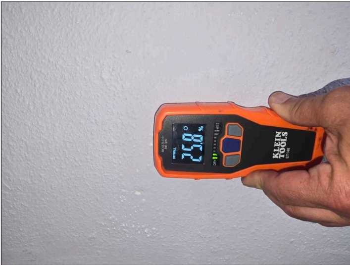
Checked water stain on the walls with a moisture meter and found to be at higher than normal moisture level. Unable to determine condition of the underlying materials. Mainly at - living room
