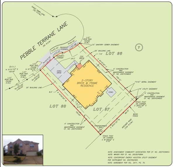
THIS PROPERTY DOES NOT LIE WITHIN THE 100 YEAR FLOOD PLAIN AS PER FIRM PANEL NO. 48157C 0105 LM PREVISION: 04/02/2014 ZONE X BASED ONLY ON VISUAL EXAMINATION OF MAPS. INACCURACIES OF FEMA MAPS PREVENT EXACT DETERMINATION WITHOUT DETAILED FIELD STUDY
