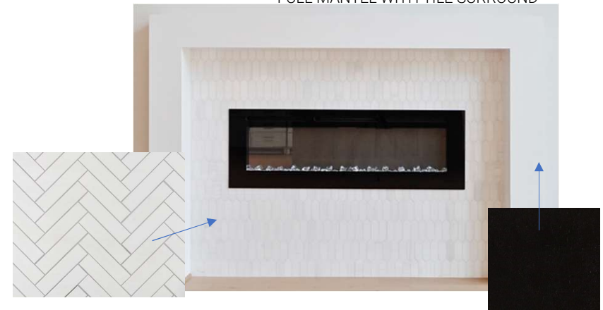
FULL MANTEL WITH TILE SURROUND
