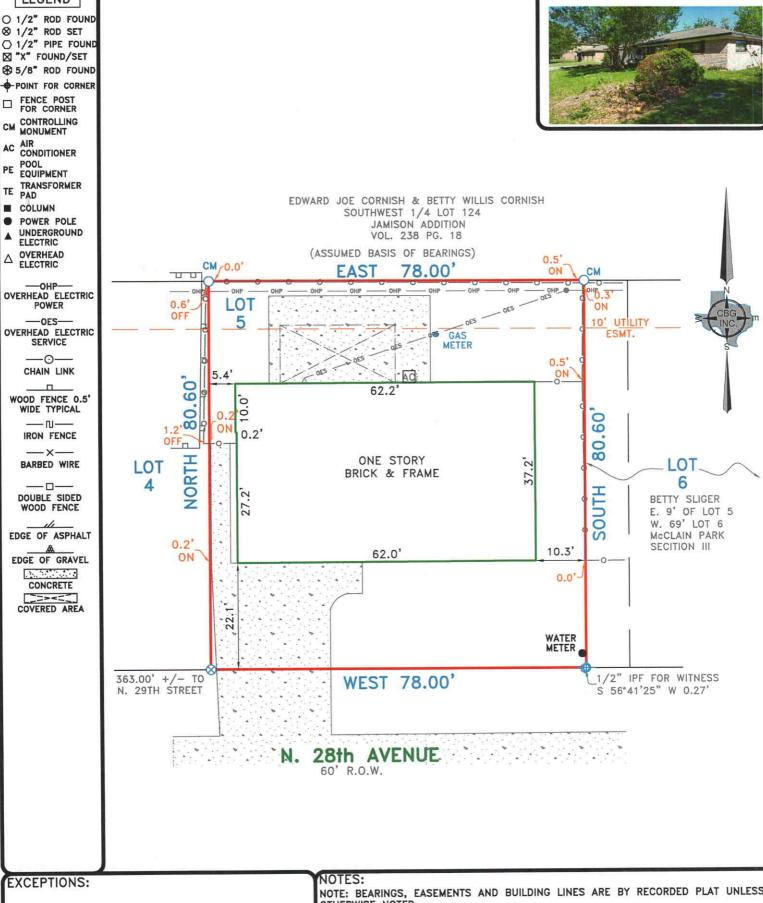
NOTE: BEARINGS, EASEMENTS AND BUILDING LINES ARE BY RECORDED PLAT UNLESS OTHERWISE NOTED.
