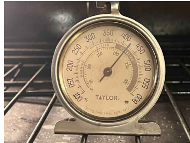
420°F (Upper Oven) – Inadequate
