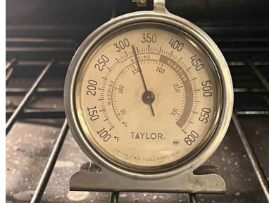
320°F (Upper Oven) – Inadequate
