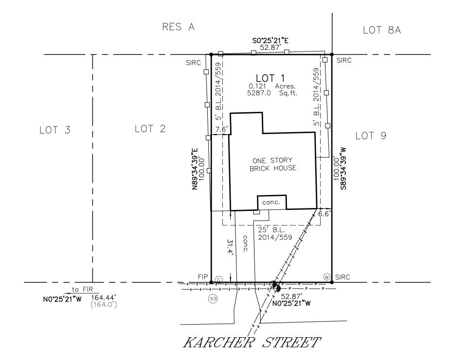
BEARING BASED ON THE TEXAS COORDINATE SYSTEM OF 1983(NAD83) CENTRAL TEXAS ZONE, BASED ON LOCAL GPS OBSERVATIONS.
