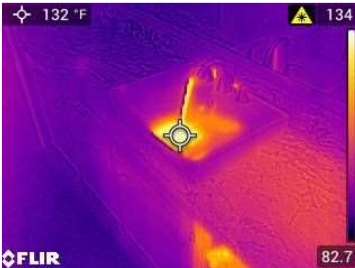
Hot water temperature - optimum - bathroom
