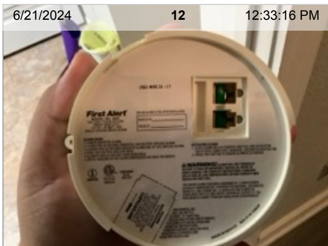
Wireless Smoke Alarm (mfd 5/2022) | Smoke test: Passed | Close-up of printed manufacture date | 2.1 years old
