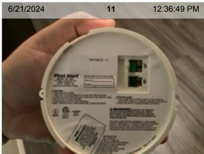
Wireless Smoke Alarm (mfd 3/2022) | Smoke test: Passed | Close-up of printed manufacture date | 2.3 years old
