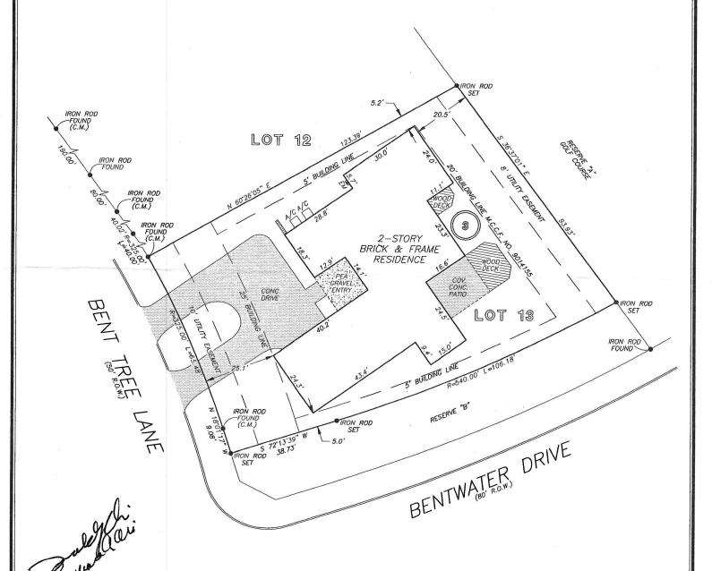
NOTE: SERVICE UTILITY EASEMENT 5' WIDE, BEING 2-1/2' ON EACH SIDE OF UNDEGROUND SERVICE LINES AS PER M.C.C.F. NO. 9014195.
