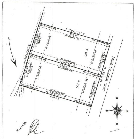
PLAT SHOWING SURVEY OF LOT 8, AND LOT 9, BLOCK ONE, OF BRIDGEPOINT SECTION ONE, ACCORDING TO THE MAP OR PLAT RECORDED IN CABINET I, SHEET 150, OF THE MAP RECORDS OF MONTGOMERY COUNTY, TEXAS, AND BEING IN THE NEIL MARTIN SURVEY A-26, MONTGOMERY COUNTY, TEXAS.
